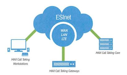
The main components of the MAX Call Taking System are: the MAX Call Taking Workstation, MAX Call Taking Core, MAX Call Taking Network Switches, and the MAX Call Taking Telephony Gateways.
